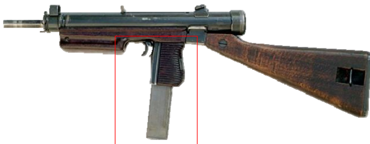
Sa 24, with fixed wooden butt, 7.62mm
