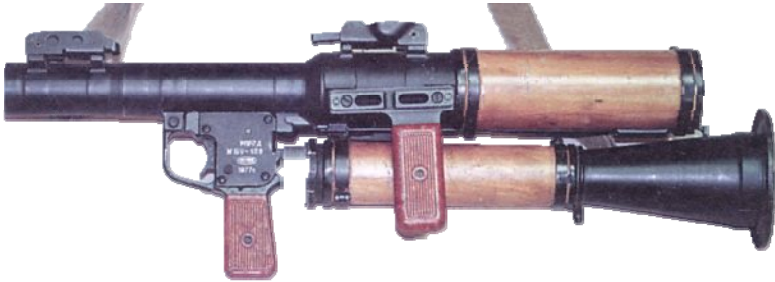
RPG-7D anti-tank grenade launcher (version for airborne troops), disassembled for transportation / airdrop
