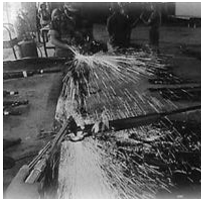
Representatives of El Salvador's Ministry of Defense destroying collected weapons using oxy-acetylene torches.
